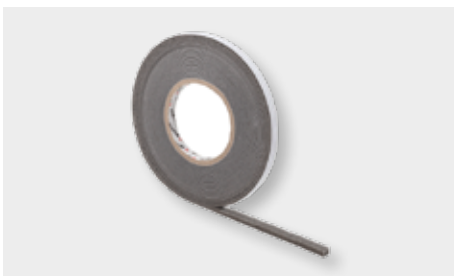
VKP® Plus sealing tape High-quality, waterproofed, pre-compressed BG1 sealing tape for secure and permanent joint sealing up to over 600 Pa • Chemical basis: fine, open-cell polyurethane foam • Sustainability: low-emission Art. no. 0875 0...
