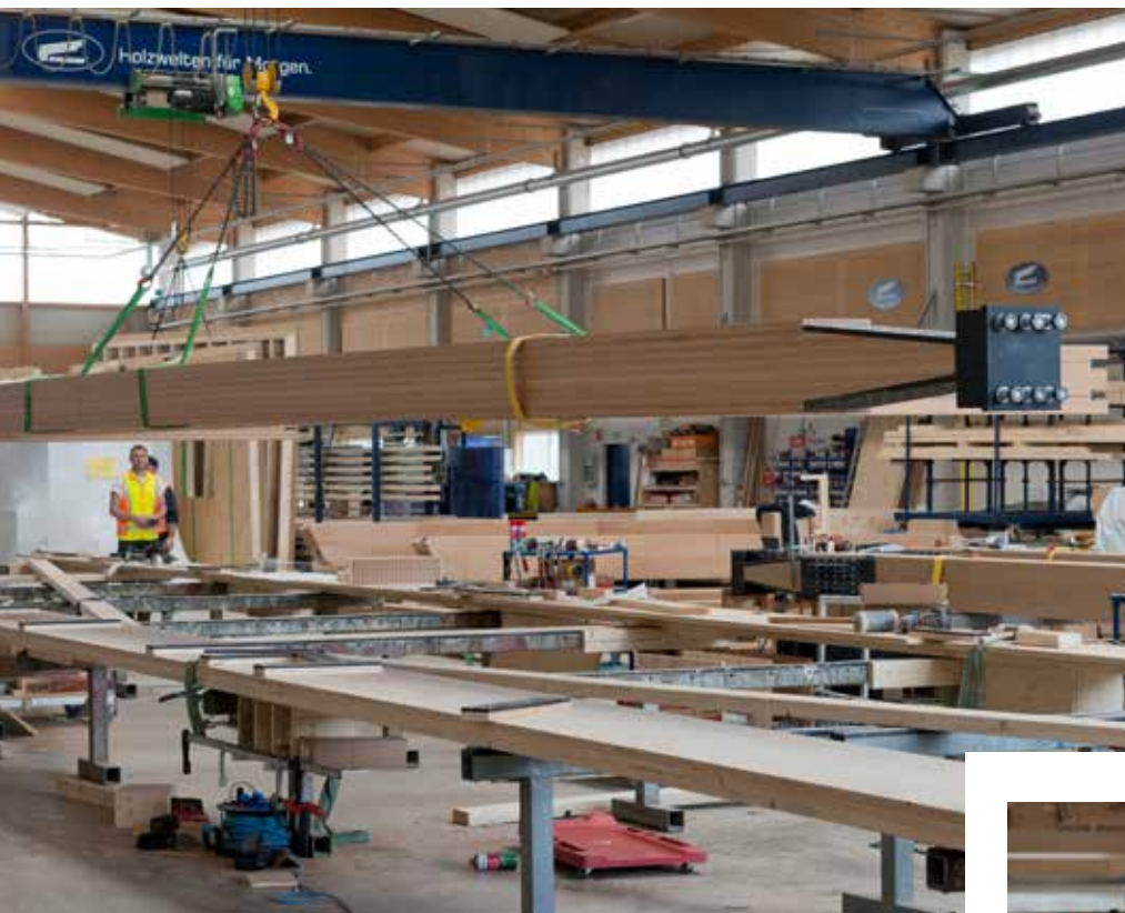
When assembling individual components, you may want to use transport systems or handling hooks. The individual components are assembled at optimum ergonomic height.
