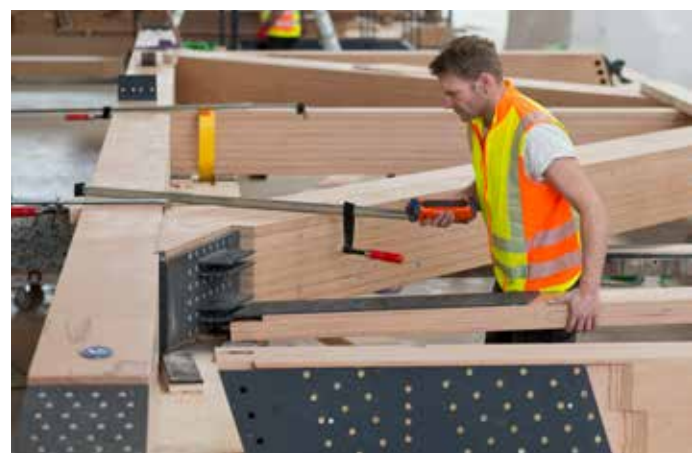
When assembling individual components, you may want to use transport systems or handling hooks. The individual components are assembled at optimum ergonomic height.
