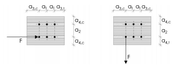
For screws in the edge surface,  $a_1$  and  $a_3$  are parallel to the CLT plane face,  $a_2$  and  $a_4$  perpendicular to CLT plane face.
