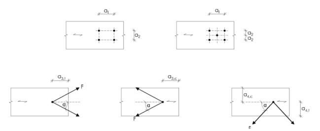
Definition of spacing, end and edge distances in the edge surface unless otherwise specified in the technical specification (ETA or hEN) for the cross laminated timber:
