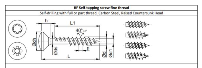
Tip: sharp, Type 17, Saw Thread and Type 17 & Saw Thread combined
