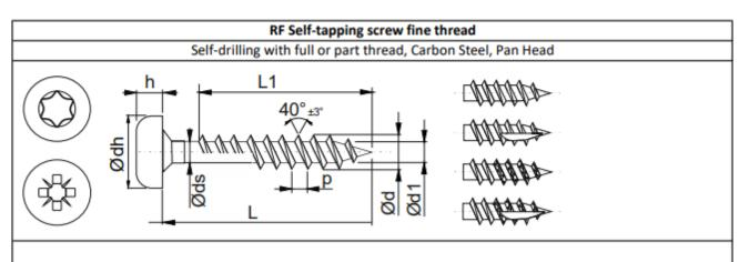
Tip: sharp, Type 17, Saw Thread and Type 17 & Saw Thread combined Shank Rips: optional for L >=25mm and d >=3,5; obligatory for L >200mm Thread Cutting Line: optional Head Mark: optional
