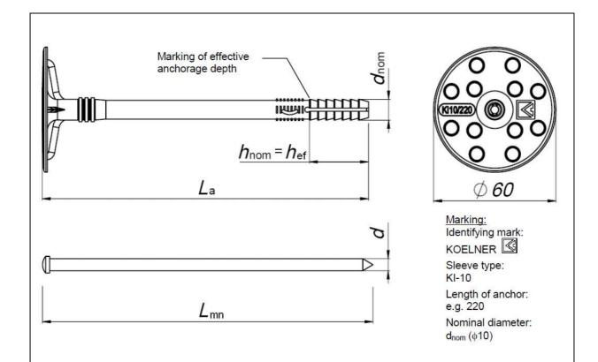
Table A2: KOELNER KI-10M anchor types and dimensions [mm]
